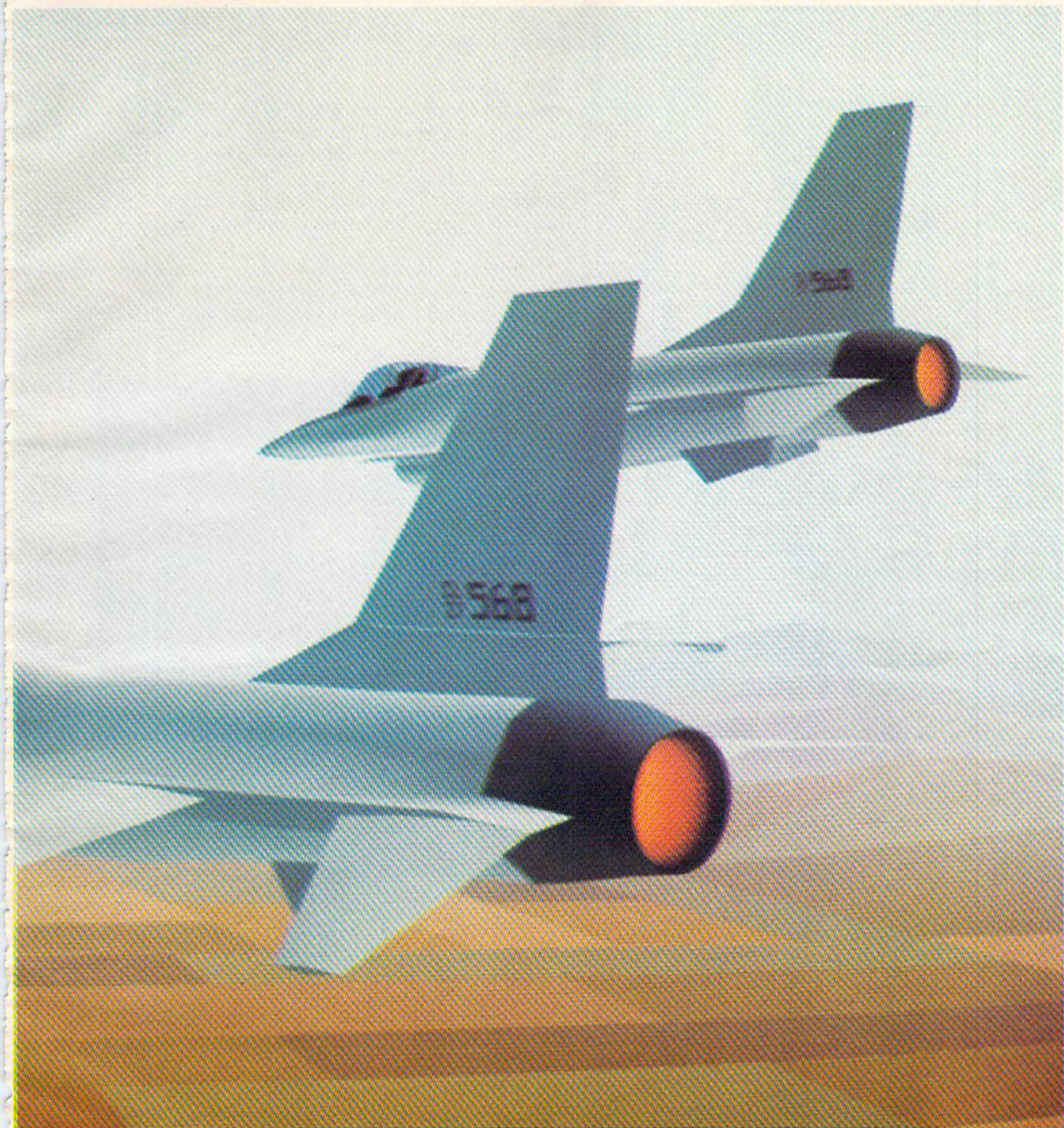
The view out the computer "window" of an Air Force flight simulator. The ultra-high resolution computer images of the jets and the ground below are in color, in 3-D, and in motion. (Courtesy Evans & Sutherland.)
